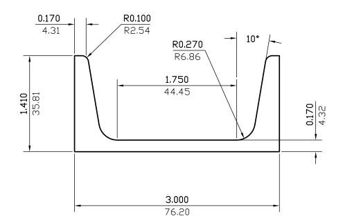
(AS SHOWN) WALL THICKNESS EXCEPT AS SHOWN DATE REV DESCRIPTION BY 03/21/23 REMOVED ALLOY NDSAL 809.811 ın.<sup>2</sup> мм.<sup>2</sup> 1.255 EST.AREA EST.AREA 2.242 1.506 EST.WT. LBS/FT. EST.WT. KG/M. 10.705 271.913 EST.PER. MM. EST.PER. OUT PER. MM. OUT PER. 3.315 C.C.D. 84.197 C.C.D. FACTOR **FINISH** M/F ALLOY & TEMP. 1:1 DWN BY L.L. DATE 11/05/2001 <u>C</u>KD BY SCALE
